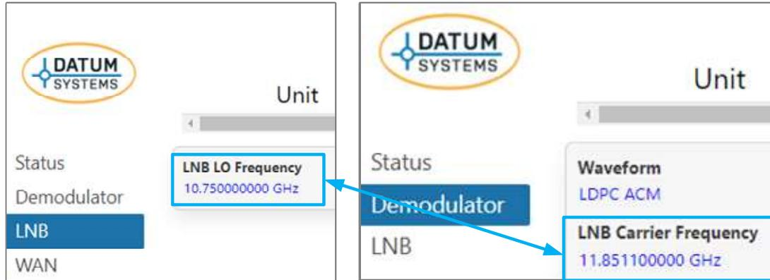
Figure 3-51 – LNB LO Frequency web page configuration
