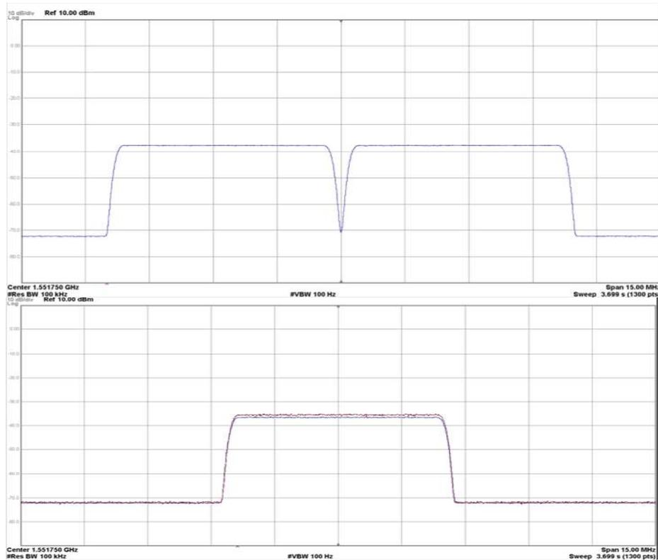
Figure 1-10 - Smart Carrier Bandwidth Savings of 50%
