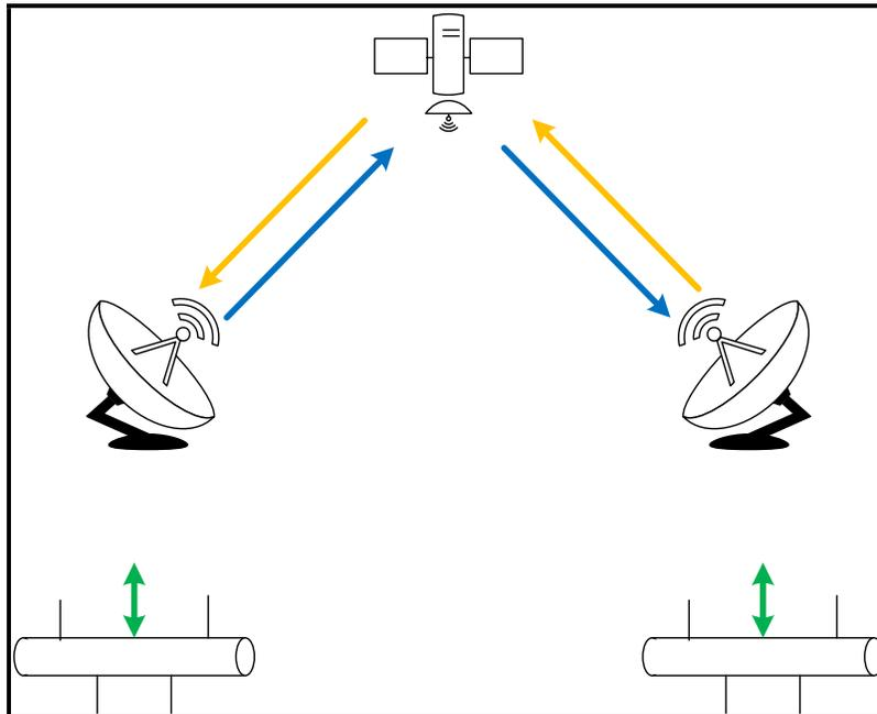
Figure 1-3 - Point-to-Point Network
