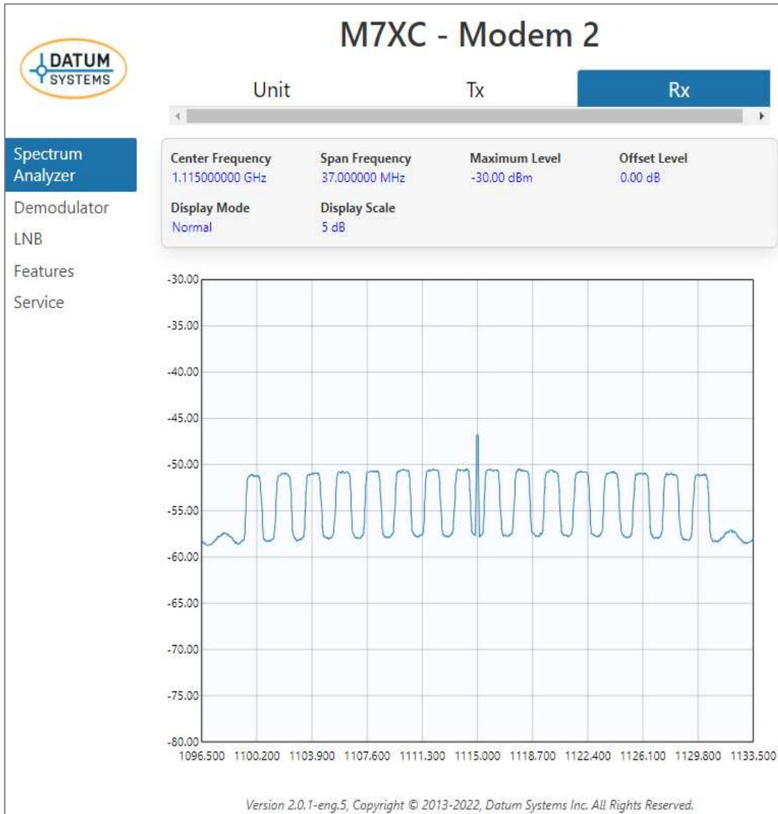
Figure 3-35 - RX Demodulator Page with Spectrum Analyzer
