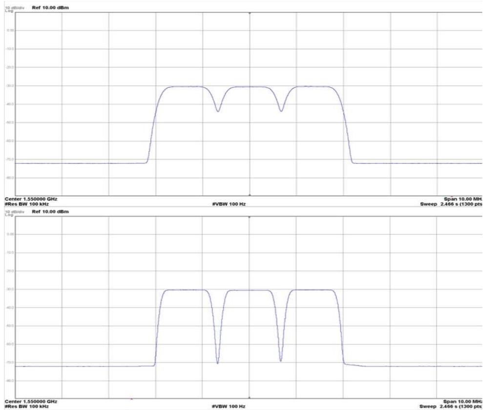
Figure 1-9 - Carrier Alpha = 0.4 vs Carrier Alpha = 0.02 Carrier Spacing
