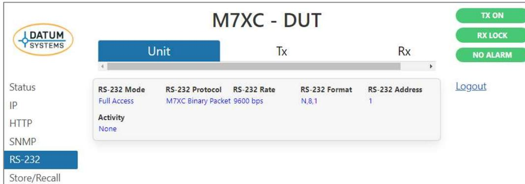
Figure 3-43 – Serial address configuration web page
