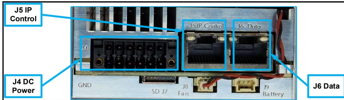
Figure 2-1 - Baseband Connections
