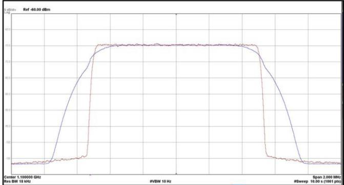
Spectrum Analyzer Plot of 0.35 versus 0.02 Roll-off factors
