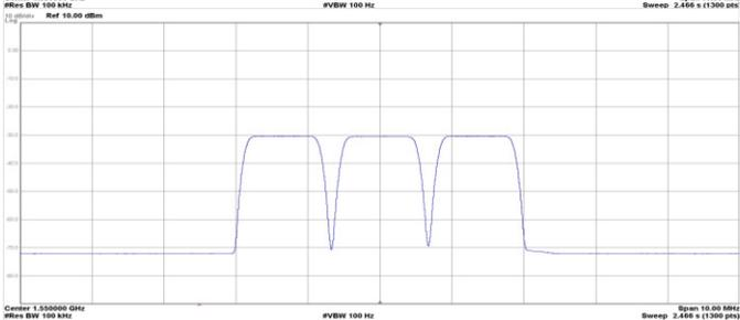
Carrier Alpha = 0.35 vs Carrier Alpha = 0.05 Carrier Spacing
