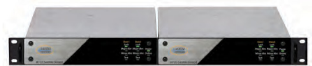
Side by Side = ACM Multi-Demod in Single Rack Unit Space
