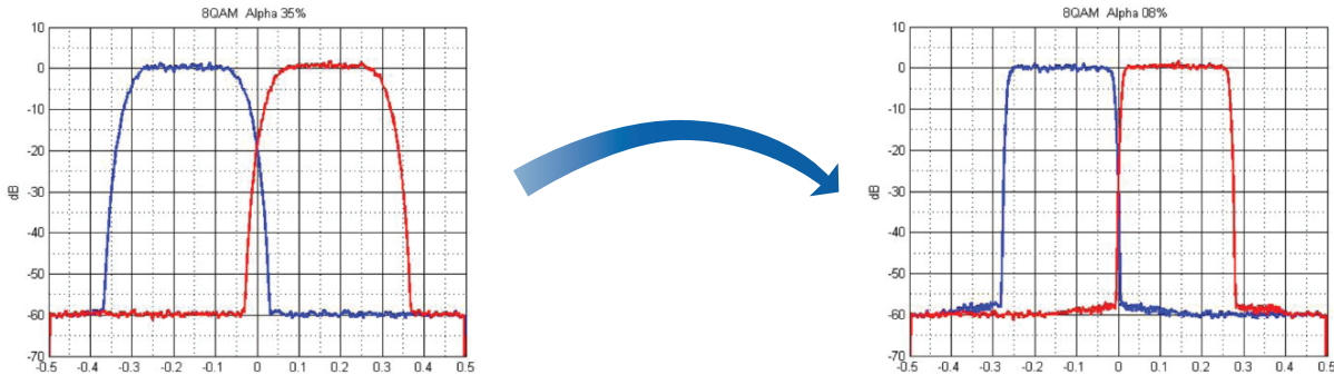
Example going from 35% to 8% Carrier Roll-Off (22% BW Savings)
