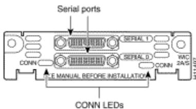
The dual serial port WIC-2T and WIC-2A/S provide higher levels of serial port density for a single WAN interface card and are supported on the Cisco 2600 and 1720 series.
