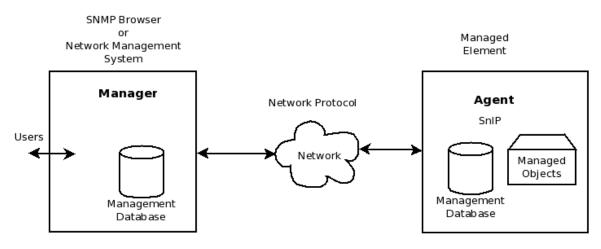
There are multiple manager end and agent end programs installed in the SnIP: The main purpose of SNMP in the SnIP is to act as an agent, returning answers to requests from a network manager station, however the standard programs installed in the SnIP include the manager programs and one Snip can act as the manager for other SnIP agents.
