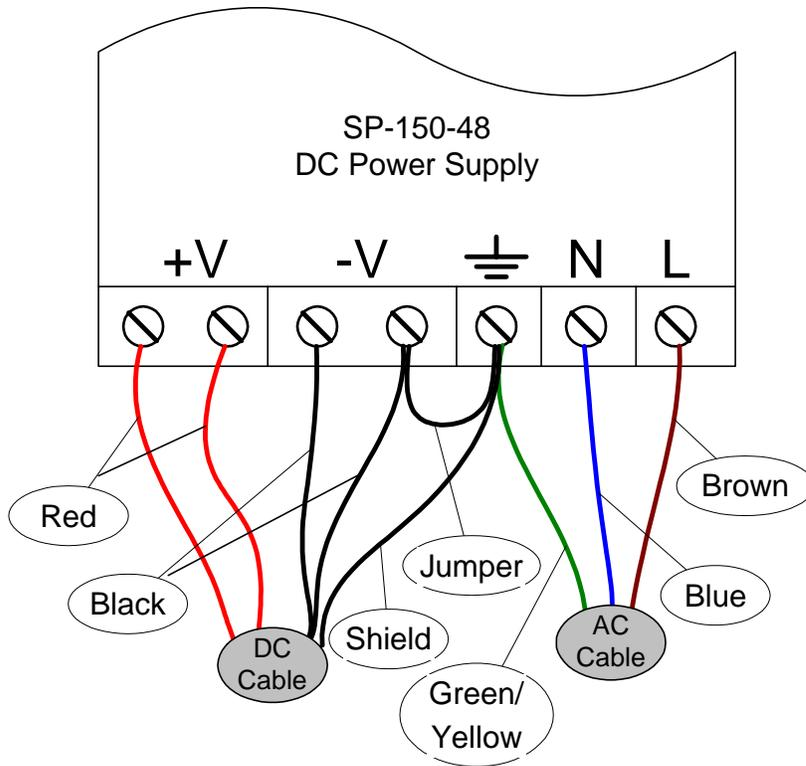
The AC cable is a 3 wire standard power cable with an AC plug appropriate for the country of use.
