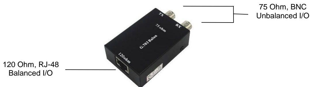
Figure 3 - Balanced to unbalanced converter (Balun)
