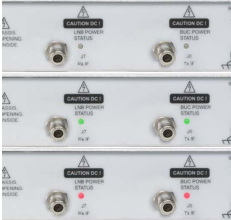
Figure 2-27 – M7LT Rear Panel indicators
