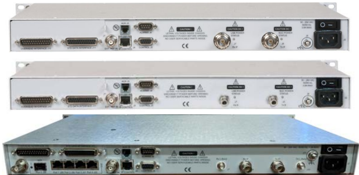
Figure 2-26 – M7LT Rear Panel Connector Options (N Type, F Type, or Dual IF)
