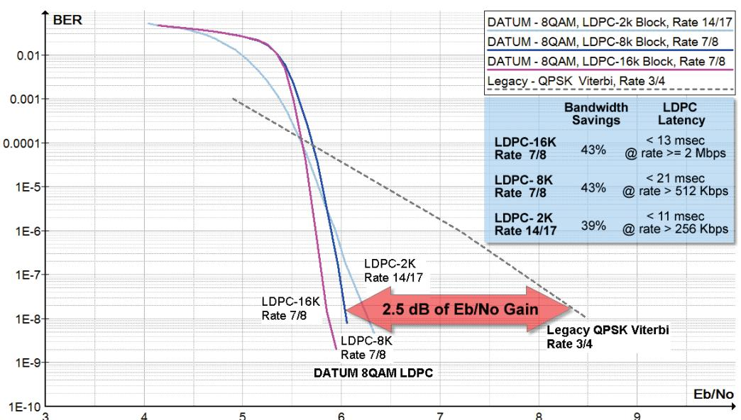
The LDPC block size can be configured to minimize processing latency for low-to-medium data rate scenarios. Thus, a 256 Kbps link can be configured with LDPC-2K block and FEC 14/17 to achieve processing latency of 11 msec, while a higher data rate link such as a 2 Mbps link can use 16K LDPC blocks with a processing latency below 13 msec. All shown coding options have equal C/N (real savings).
